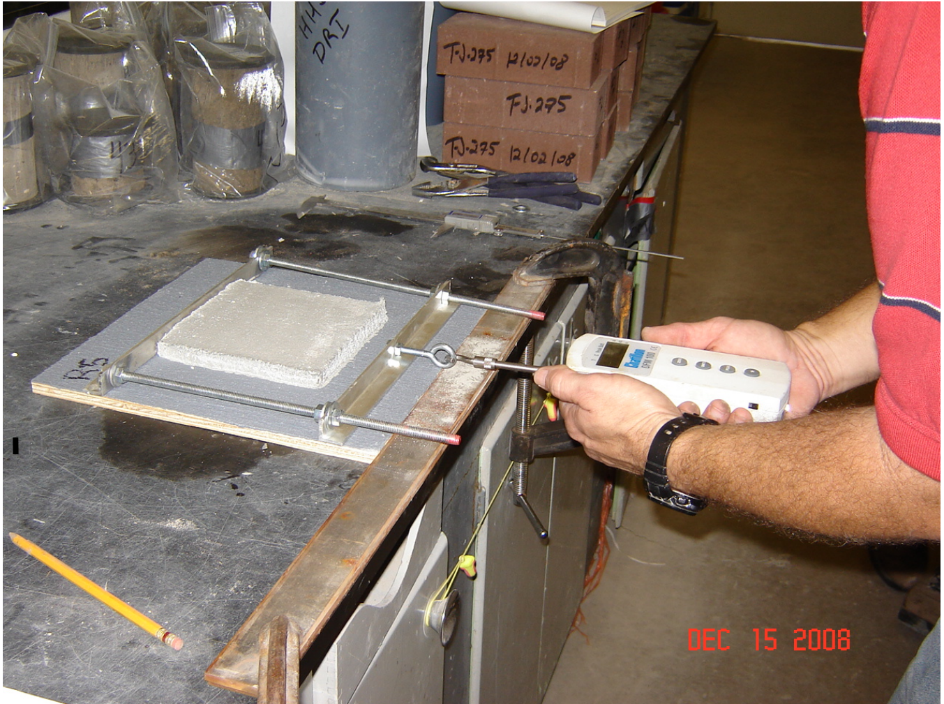
FIGURE NO. 2—DETRIMENTAL MOVEMENT TEST
