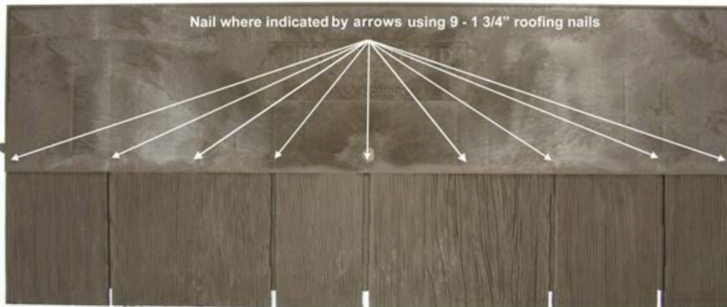
FIGURE 2—FASTENER LOCATIONS
