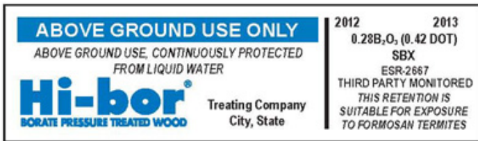
FIGURE 3—TYPICAL HI-BOR® BRAND BORATE PRESSURE TREATED STAMP DESIGN (0.42 DOT)
