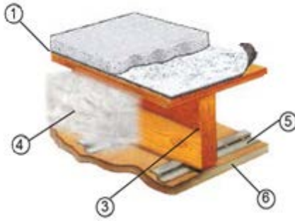
FIGURE 3—SOUND RATED ASSEMBLY INCORPORATING WOOD JOISTS
