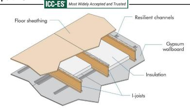
FIGURE 4—ONE-HOUR FIRE-RESISTANCE-RATED FLOOR-CEILING ASSEMBLY (Ceiling—one layer of <sup>3</sup>/<sub>4</sub>-inch Type X gypsum wallboard)
