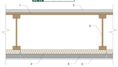
FIGURE 3—ONE-HOUR FIRE-RESISTANCE-RATED FLOOR-CEILING ASSEMBLY (Ceiling—one layer of ½-inch or 5/8-inch gypsum wallboard, attached to furring channels spaced 24 inches on center)
