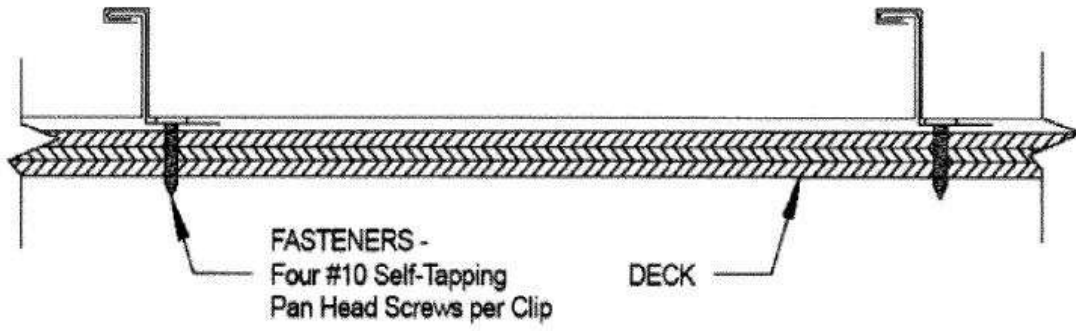
FIGURE 3—PANEL WITH CLIP AND FASTENERS
