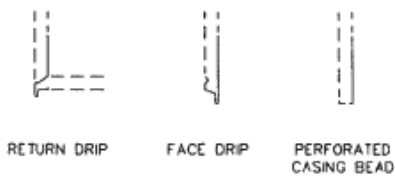
FIGURE 2—TYPICAL DETAILS FOR PERMACOAT AND UNICOAT FIBERGLASS STUCCO SYSTEMS
